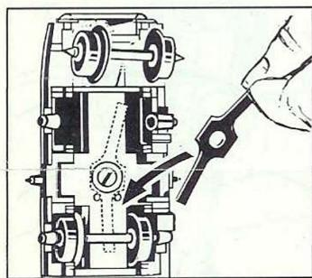
**ATTENTION!** The bulb 9530 must be replaced with bulb 6 9530 to be compatible with FMZ operation.
